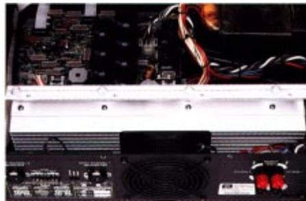
*Oversized heatsinks and powerful multiple-speed cooling fans increase reliability and maintain stable, consistent performance. This outstanding cooling capability allows MPX Series to deliver power continuously in high ambient temperature environments or into low impedance loads longer than most other amplifiers.*
