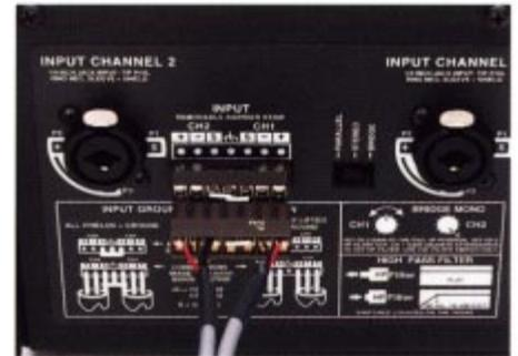
*In addition to balanced or unbalanced XLR and 1/4 inch TRS phone jack connectors, we also provide a barrier strip which is removable, making it possible to make all hard-wire connections on a workbench rather than behind a dark cramped equipment rack.*
