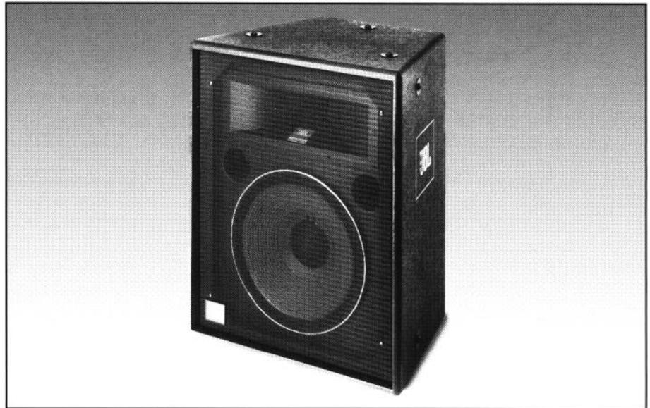
The 2426H compression driver used in the AS4725 incorporates a pure titanium diaphragm that is both light and strong. It has a three dimensional embossed pattern which controls high frequency resonances and results in usable response to 18 kHz. The 2370A Flat-Front Bi-Radial® horn provides a tightly controlled radiation pattern.
