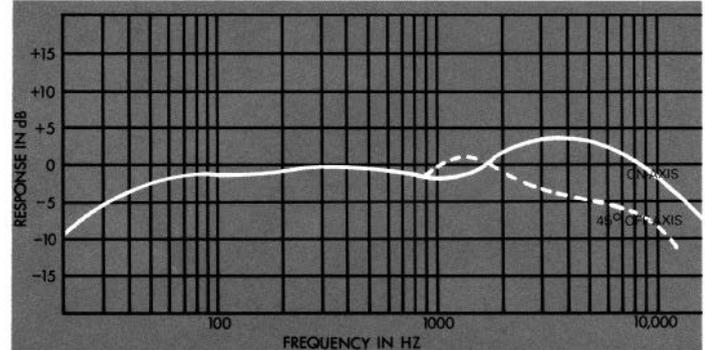
Frequency response contour of the 2115 in a closed box of 170 L (6 ft<sup>3</sup>) internal volume. Measured response of a typical production unit, including all peaks and dips, does not deviate more than 2 dB from the above curve. Additional acoustic loading (a port) will further extend bass response.
